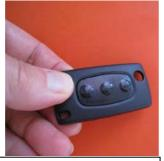
Next press fit your new key pad in the top cover. No gluing is required. Once key pad is in, put your remote together in reverse order and close it.
