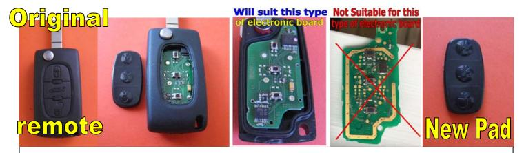
Silicone Replacement Pads from POLMEX for worn flip Peugeot remotes with 2 buttons or 3 buttons.
