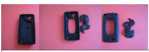
You have to make sure that grooves around cut out are free from old rubber remnants before you press fit new pad in.
