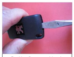
Position flat screwdriver in a small slot located at the bottom
