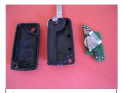
Separate electronic board from top part of your remote in preparation for removing an existing plastic key pad.
