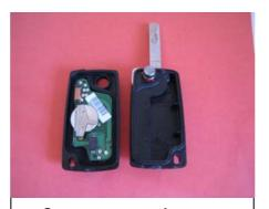
Separate parts of your remote. One part consists of key blade and top part with key buttons and electronic board.
